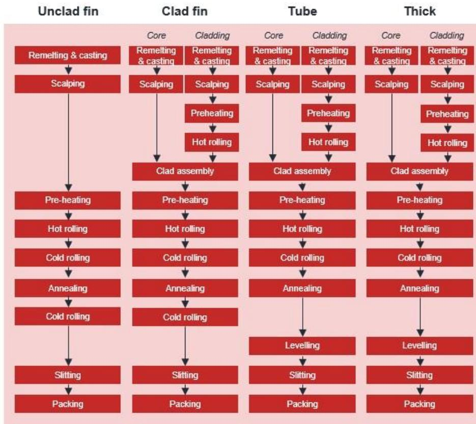
Figure 4. Process routes for different products.
