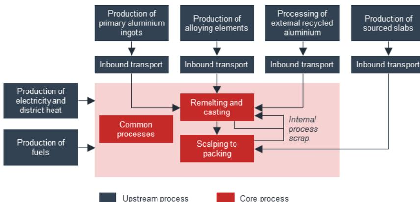
Figure 2. Generic flow chart for upstream (blue) and core (red) processes.
