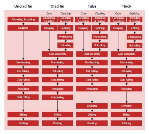
Figure 4. Process routes for different products.
