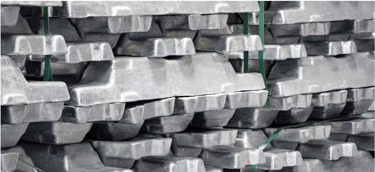
Primary aluminium slabs and ingots (see image) serve as input material for Gränges' production.
